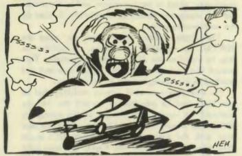
HOW TO RUIN A CANOPY. Immediately after the pilot locked the canopy of a T-bird the cockpit started pressurizing at an abnormal rate causing discomfort to both occupants. The temperature control was placed to full cold to minimize the pressure, but this had no effect. The pilot then unlocked the canopy and the whole works blew upward approximately 8 to 12 inches, the drive chains broke, and the canopy fell back onto the cockpit rails.
